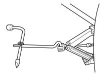
To lessen the risk of personal injury, do not put any part of your body under the vehicle while changing a tire. Do not start the engine when your vehicle is on the jack. The jack is only meant for changing the tire.
